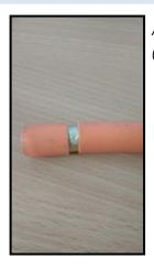
A ring slit on a 15 mm (0.59") Coroplast cable
